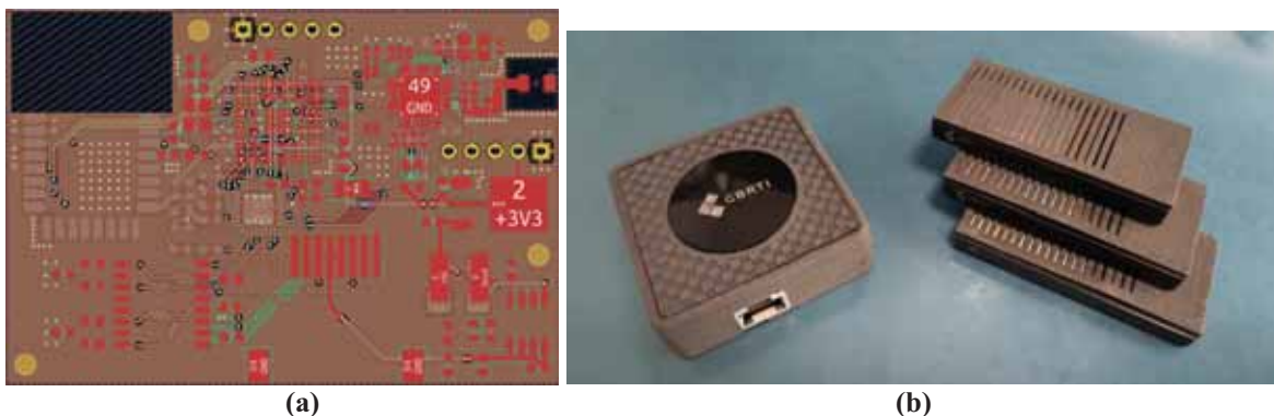
Fig. 1. Author's coupling solutions created in the project: (a) – mosaic of electrical connections of the ultra-wideband anchor, (b) – actual prototypes of the UWB anchor (left) and UWB tags (right)
