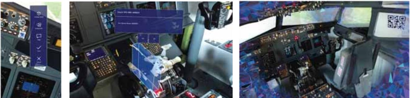
**Figure 3.** The screenshot of VRM pilot training system. On the left picture there is shown defining flight procedure by admin, on the middle one, the realization of the “aircraft structure and equipment” training. On the right one – the localization and QR recognition for calibration of the system.
