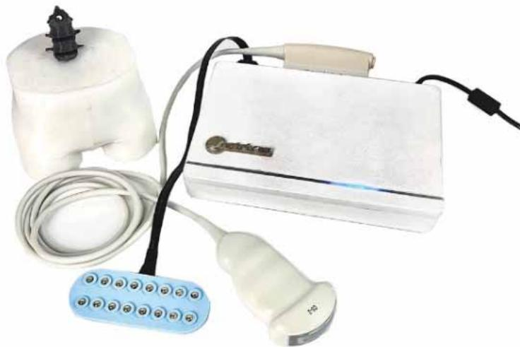
**Fig. 1.** Photo of EIT-UST hybrid tomograph. The device is equipped with an ultrasonic head and a set of measuring electrodes
